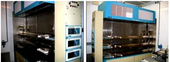
During a run the temperature is ramped from a low temperature (900°C) to the oxidation temperature. A description of of each interval for the recipe of trans-LC dry oxidation is given below.
